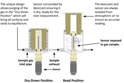
Keeping the sensor dry between tests ensures that the SDHmini-Ex is ready to carry out rapid spot checks. The unique design of the desiccant head achieves this by surrounding the sensor with desiccant, keeping the sensor dry. The head is then lifted for sampling, exposing the sensor to the sample gas.
